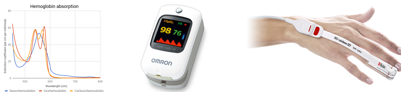
Figure 1. (Left) The spectrum for deoxyhemoglobin, oxyhemoglobin, carboxyhemoglobin, and methemoglobin. These curves offer multiple isosbestic points and also require measurement at points of mutual separation for effective measurement; multiple wavelengths are required to separate these variants. (Center) A consumer pulse oximetry product produced by Omron (Right) A typical medical-grade oximeter module, showing the Rainbow SET from Masimo.
