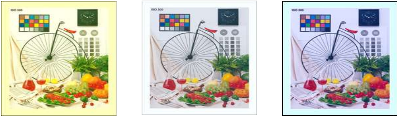
Figure 1. Example of white point modification to match the ambient white point.[4] Viewers accommodate to the white point in the environment, and colors in a display appear incorrect when seen after adaptation to a white point different from the display's reference. Adjustment of the color space to the ambient white point matches this accommodation, yielding a perceptual match of the images shown on the display independent of the environment.
